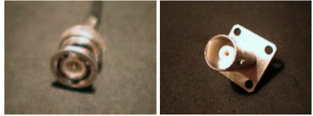
BNC plug and socket
