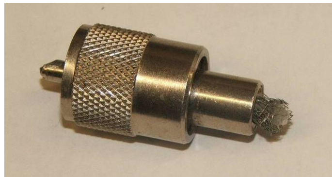
Photo 2 – The clean cut right through the Coax.
